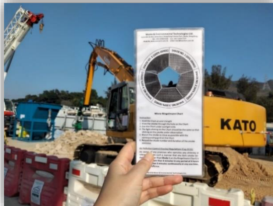
定期檢查機械以確保機械沒有排放黑煙 Plants were checked regularly against Ringelmann Chart to ensure no emission of dark smoke
