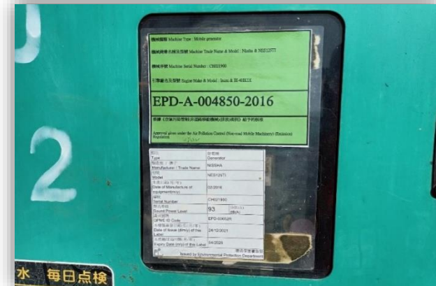
使用合乎環保署訂明的廢氣排放標準的非道路移動機械 Adopted EPD approved non-road mobile machinery system which complies with prescribed emission standards
